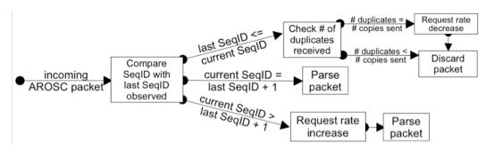
Figure 2 – AROscRecv handling incoming packets
